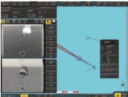
AIS and automatic radar plotting aid (ARPA) targets are plotted on the same chart, which makes it possible to monitor all the traffic surrounding the operations.
